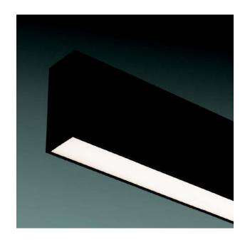
The Linear Rigel is an LED luminaire made of an extruded aluminium, powder-coated with a fine matte finish providing a direct light through a PMMA diffuser. Available as a ceiling mounted, recessed, trimless or suspended fitting, the Linear Rigel is available in Black or White finishes and various lengths.
